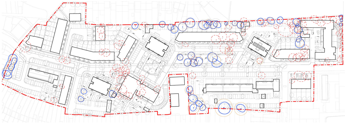
Existing tree removal / retention plan
