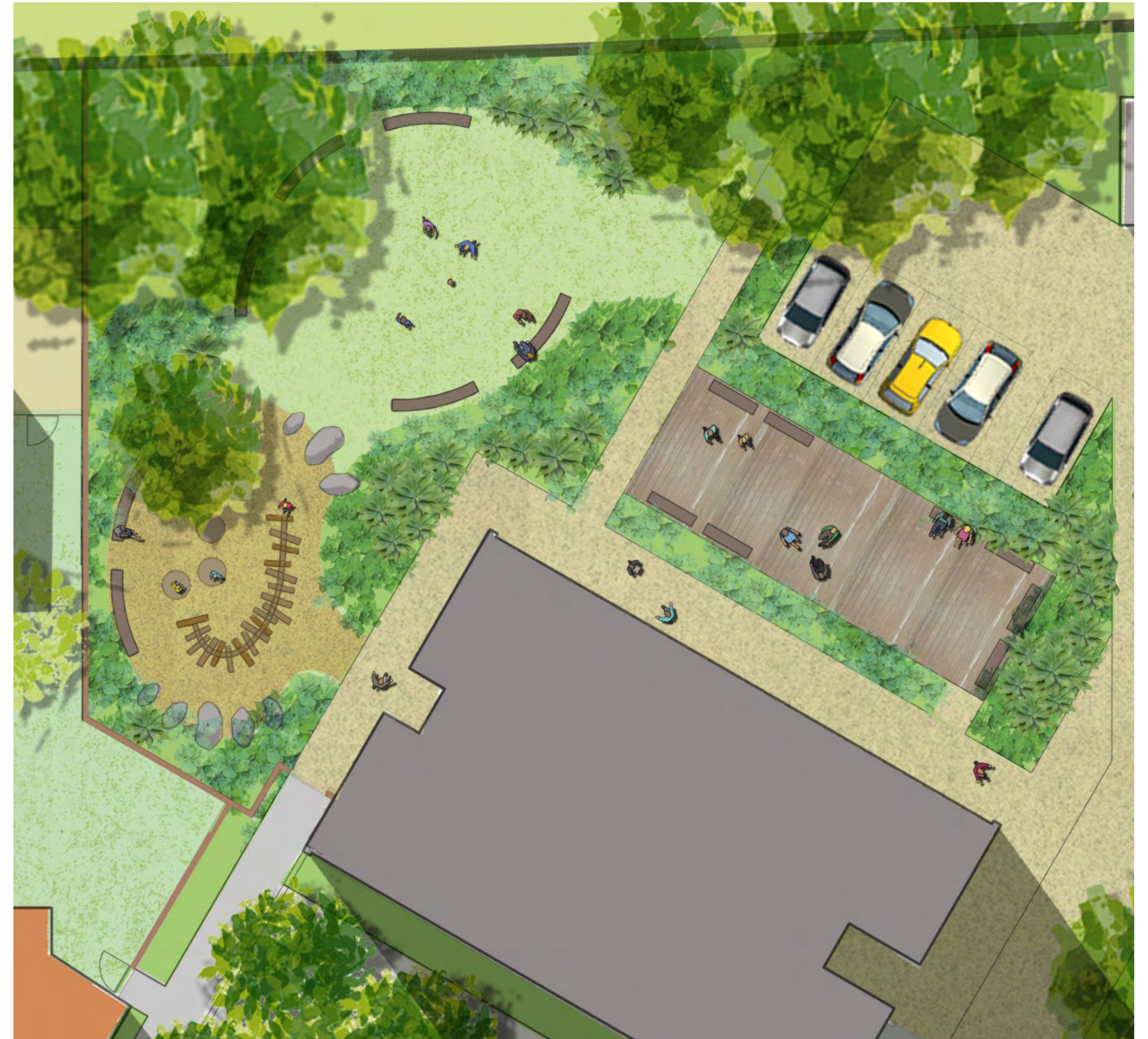
Detail plan to show the design of a typical communal garden for each tower
